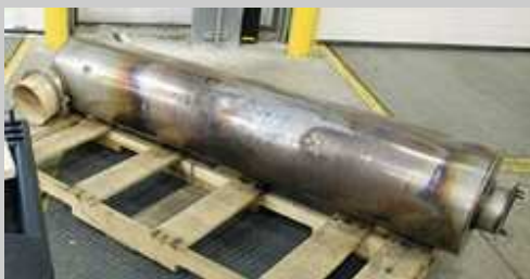
Energy Logic's light weight blast tube.
