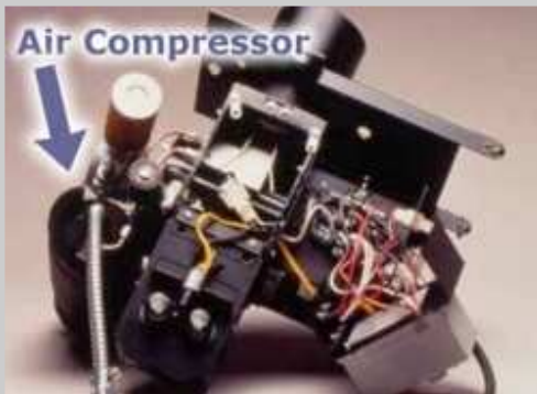
Air compressor included -- considered noisy by some and a potential maintenance issue.
