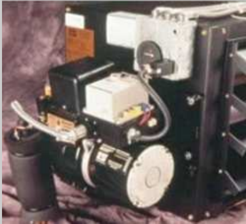
Modified Becket #2 oil burner converted for waste oil which makes for increased maintenance.
