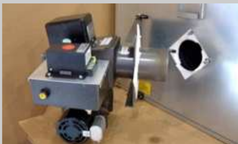
Swing out burner design necessitates disconnection of oil and air lines.
