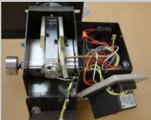
The complicated design of the Lanair burner and pre-heater block may make serviceability difficult. The burner has an electric air solenoid valve that acts as a shut-off valve, but is located inside the burner's electrical box, making service difficult.
